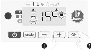
If you do not want to change it, press **OK**: the device changes automatically to set the maximum setting. To exit the user settings, press **mode** twice.
