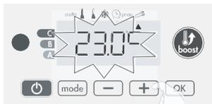
To validate, save the new value and exit the mode, press (OK). To exit the Expert settings, press (mode) 3 times.
