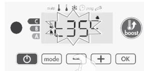
13- To save and move automatically to the next setting, press **OK**. To exit the user settings, press **mode** twice.
