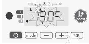
**Note:** The cursor corresponding to the operating mode, i.e Eco mode in our example, is blinking during the duration of the temporary derogation.
