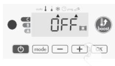
2- To save and move automatically to the next setting, press **[OK]**. To exit the user settings, press **[mode]** 3 times.
