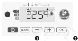
To save and move automatically to the next setting, press [OK]. To exit the user settings, press [mode] twice.
