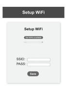
Click on the drop-down menu (---) to display the names of the networks (SSIDs) that have been found in the environment and select one. You can also enter the name of the network directly in the "SSID" field.
